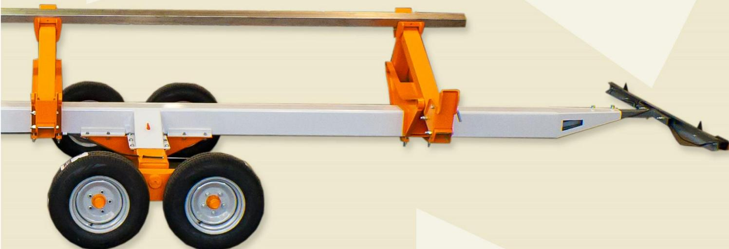
To assemble the trailer, it is sufficient to screw the axel to the central frame.
